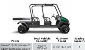
With four forward-facing seats, a higher ground clearance and standard all-terrain tires for the ultimate in passenger comfort. IntelliTrak also standard.
